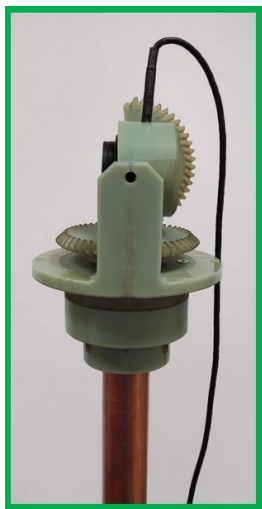
Figure 2. Goniometer with mounted detector in vertical measurement state
