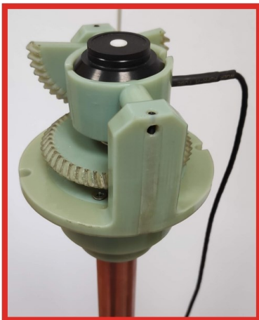
Figure 1. Goniometer with mounted detector in horizontal measurement state
